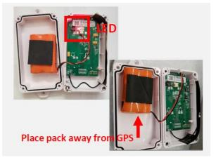
**Step 6:** Replace the top cover and ensure top and bottom are aligned before closing the device and securing with screws.
