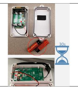
**Step 5:** Replace the batteries – LED should flash for a second, indicating the device is powered up. Ensure the batteries are placed properly and match the + and – outlined on the device board. Ensure the foam pad is sandwiched between the battery pack and the board and that the battery pack is at the top of the board to avoid obstructing the GPS.
