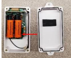
**Step 3:** Carefully unhook the cable linking the battery pack from the board.
